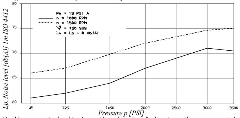
*Double pump noise level is given with each section discharging at the pressure noted on the curve.*
