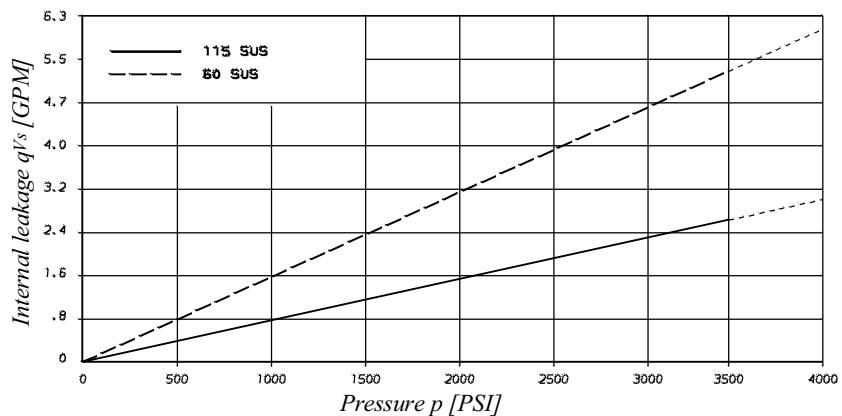
*Do not operate pump more than 5 seconds at any speed or viscosity if the internal leakage is more than 50% of the theoretical flow.*
