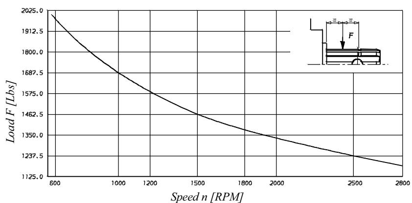
*Life time 3000 hours when 70% of the time at 500 N and 30% at max. load.*
