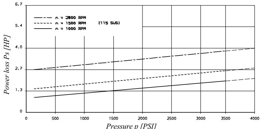
*Total hydrodynamic power loss is the sum of each section at its operating conditions.*
