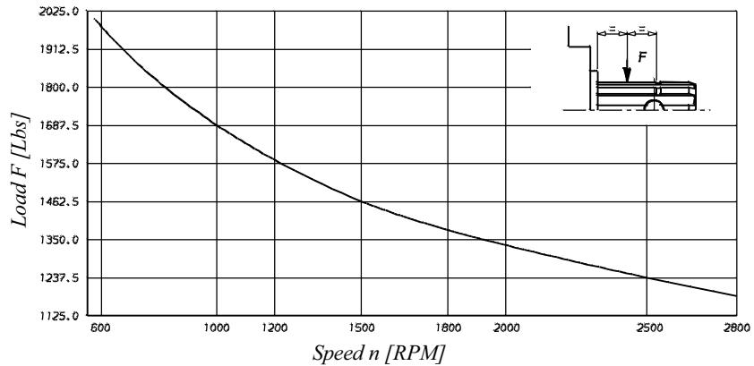
*Life time 3000 hours when 70% of the time at 112 Lbs and 30% at max. load.*
